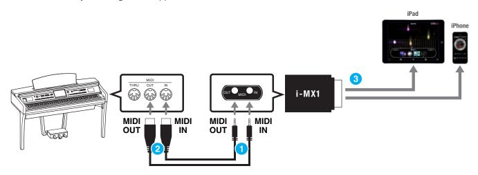
Please make sure that i-MX1 MIDI OUT terminal is connected to the MIDI IN terminal of the instrument, and the i-MX1 MIDI IN terminal to the MIDI OUT terminal of the instrument.
