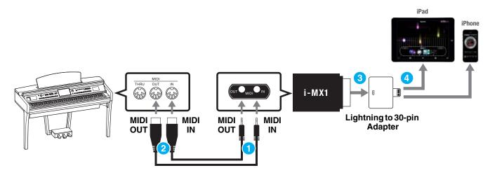
Please make sure that i-MX1 MIDI OUT terminal is connected to the MIDI IN terminal of the instrument, and the i-MX1 MIDI IN terminal to the MIDI OUT terminal of the instrument.
